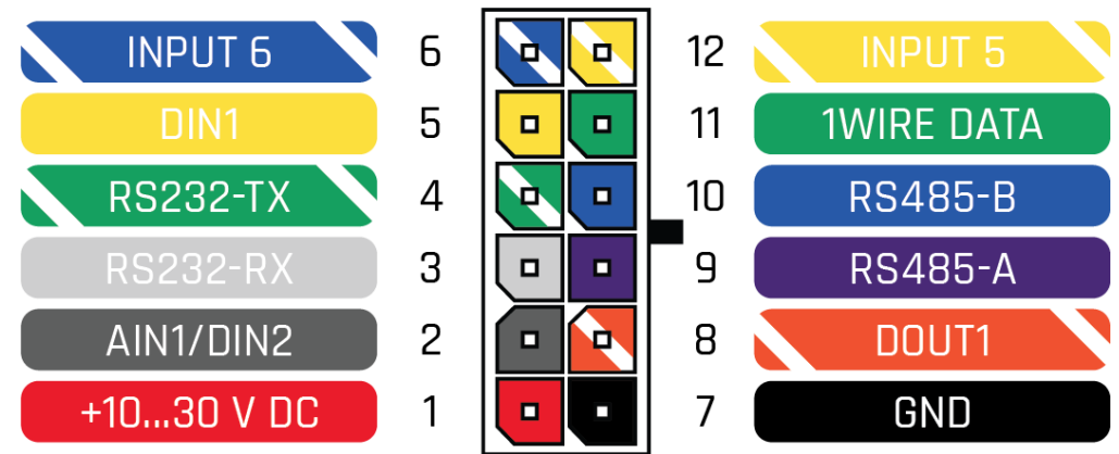
Figure 2 FMC125 2x6 socket pinout
