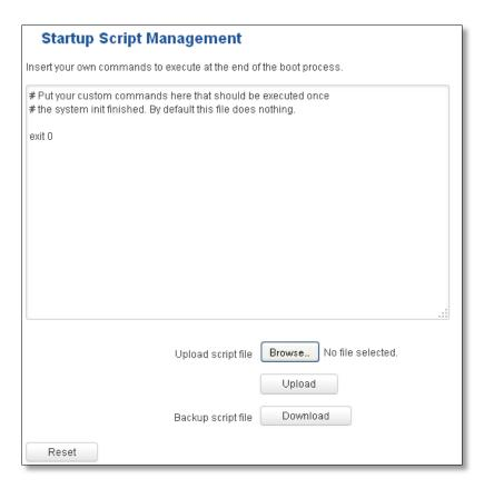
In *Script Management* window is shown content of a file /etc/rc.local. This file is executed at the end of startup, executing the line: sh /etc/rc.local In this script is needed to use sh (ash) commands. It should be noted, that this is embedded device and sh functionality is not full.
