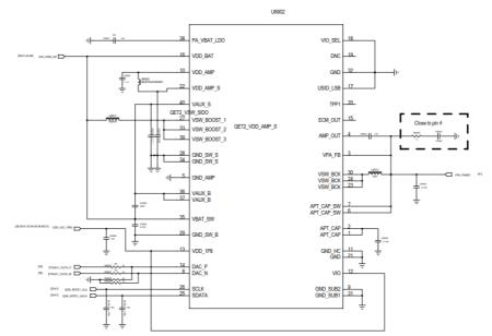
The supply VBAT (pin C2) is from VPH\_PWR, which is changed from the battery voltage. Refer to the figure as above, the maximum output voltage (pin 1 &2) is 5V during normal operation, and the specification of chips U6900/U6902 shows the maximum permitted output voltage is 5.5V,
