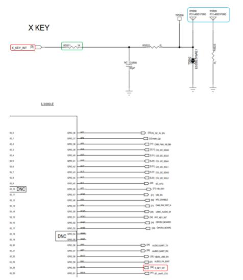
The X button is supplied from pin GPIO\_60 of chip U1000-F through a resistor R5511 (1K $\Omega$ , 5%) (Refer to drawing "EX-9900-07-01", sheet 5 & 34), the maximum voltage into the X key is less than the battery voltage 4.45V, so the maximum available current to the X key under normal operation is 4.45Vdc/ [(1000\*0.95)] =4.65mA. This is significantly lower than the limitation according to IEC 60079-11:2011 Table A.1 for level of protection 'ic' with safety factor 1.0.
