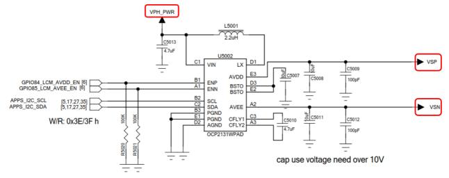
The supply VIN (pin C1) is from VPH\_PWR, which is changed from the battery voltage. Refer to the figure as above, the maximum voltage of output between the pin VSP (AVDD) and VSN(AVEE) is 10V during normal operation. And the datasheet of U5000 specified that the maximum voltage between the pin VSP (AVDD) and VSN(AVEE) is 12V.
