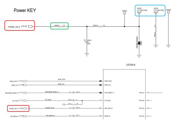
The Power button is supplied from pin 23 of chip U2100-A through a resistor R5500 (1K $\Omega$ , 5%) (Refer to drawing "EX-9900-07-01", sheet 12 & 34), the maximum voltage into the power key is less than the battery voltage 4.45V, so the maximum available current to the power key under normal operation is 4.45Vdc/ [(1000\*0.95)] =4.68mA. This is significantly lower than the limitation according to IEC 60079-11:2011 Table A.1 for level of protection 'ic' with safety factor 1.0.
