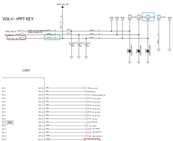
The PPT button is supplied from pin GPIO\_51 of chip U1000-F through a resistor R5510 (1K $\Omega$ , 5%) (Refer to drawing "EX-9900-07-01", sheet 5 & 34), the maximum voltage into the PPT key is less than the battery voltage 4.45V, so the maximum available current to the PPT key under normal operation is 4.45Vdc/ [(1000\*0.95)] = 4.68mA. This is significantly lower than the limitation according to IEC 60079-11:2011 Table A.1 for level of protection 'ic' with safety factor 1.0.
