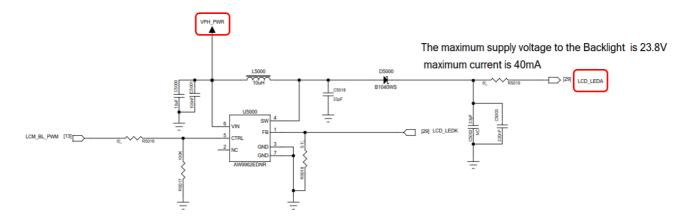
The supply VIN (pin 6) is from VPH\_PWR, which is charged from the battery voltage. Refer to the figure as above, the maximum voltage of output SW (pin 4) is 23.8V during normal operation. And the datasheet of U5000 specified that the maximum voltage on SW (PIN 4) is 40V.
