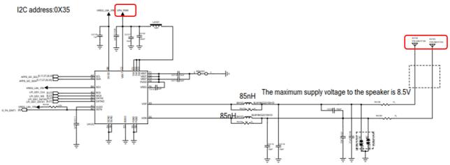
The supply VBAT (pin C2) is from VPH\_PWR, which is changed from the battery voltage. The maximum voltage to speaker is 8.5V during normal operation. The specification of the U4100 shows the maximum permitted voltage of output is 13V.
