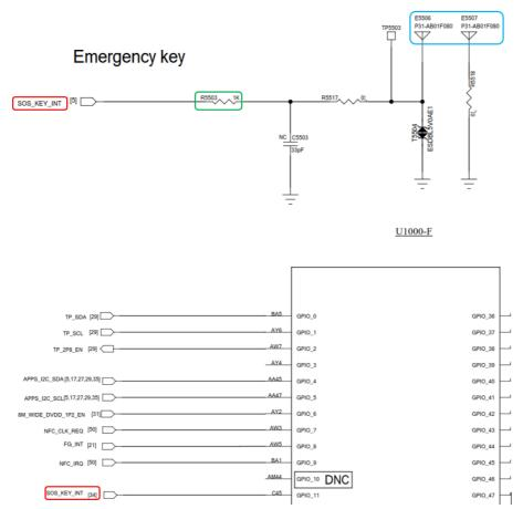
The Emergency button is supplied from pin GPIO\_11 of chip U1000-F through a resistor R5503 (1K $\Omega$ , 5%) (Refer to drawing "EX-9900-07-01", sheet 5 & 34), the maximum voltage into the Emergency key is less than the battery voltage 4.45V, so the maximum available current to the Emergency key under normal operation is 4.45Vdc/ [(1000\*0.95)] =4.65mA. This is significantly lower than the limitation according to IEC 60079-11:2011 Table A.1 for level of protection 'ic' with safety factor 1.0.
